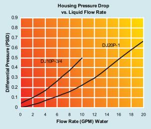
\* For liquids other than water, multiply the pressure drop by the specific gravity of the fluid.
