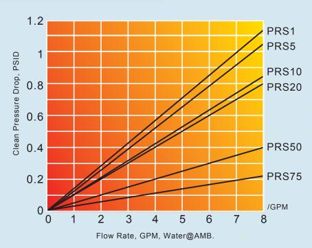
Flow rate is per 10" cartridge. For liquids other than water, multiply the pressure drop by the fluid viscosity in centipoises
